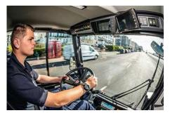
All functions of the washing unit are controlled via the door control panel with various joysticks and push buttons. The most important information is visible at a glance on the colour display in the roof console. In addition, a mechanic can make machine-specific settings in the display. With the aid of the onboard diagnosis system, any faults can be localised quickly and efficiently.
