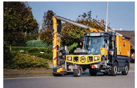
The **Cleango 500 SKR** has a fresh water volume of 685 l and thus enables long working hours. Optionally, the water volume can be expanded via additional tanks.
