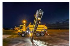
The solid parallelogram construction at the front of the machine ensures safe guidance of the spraying arms. The outer spraying arm sections are made of aluminium and have collision protection through a break-out system.
