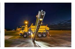
The solid parallelogram construction at the front of the machine ensures safe quidance of the spraying arms. The outer spraying arm sections are made of aluminium and have collision protection through a break-out system.
