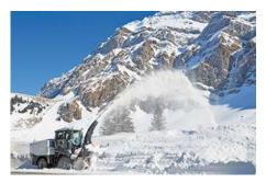
The high-capacity Supra 5002 can be equipped with hydraulically movable front flaps especially for use at airports. This increases the clearing width and can be flexibly adapted to the width of the snow bank, allowing particularly efficient snow removal. In addition to its great clearing efficiency, the Supra's all wheel drive makes it highly manoeuvrable very important in narrow areas on airports and near aircraft.
