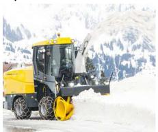
The Supra 4002 is a self-propelled snow clearing machine with a clearing width of either 2400, 2600 or 2800 mm.
