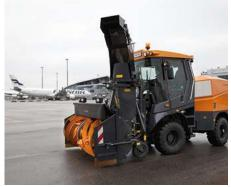
The Supra 5002 is a self-propelled snow clearing machine with a clearing width of either 2400, 2600 or 2800 mm.
