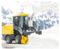
The Supra 4002 is a self-propelled snow clearing machine with a clearing width of either 94.5, 102.4 or 110.2 in.
