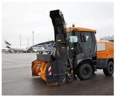
The Supra 5002 is a self-propelled snow clearing machine with a clearing width of either 94.5, 102.4 or 110.2 in.
