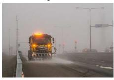
The electric hose reel and all the nozzles of the SCW street washer are located at the front washing head, which is mounted onto a front attachment of the carrying truck without any additional lifting equipment. The washing head has a lifting device to adjust the impact force from the jets to the road surface and the working width.
