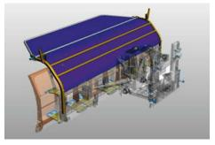
3. an adjustable snow deflector made of cloth. This version is particularly suitable for powder snow and high speeds. A combination with the polyurethane or rubber snow deflector is possible.
