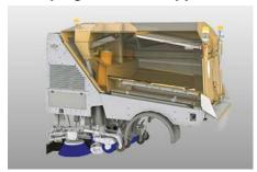
The large 7.0m<sup>3</sup> hopper allows for the collection of large quantities of debris. The floor pan made from stainless steel and the rubberised baffle plates inside the hopper combine to ensure a lengthy service life and virtually no wear.
