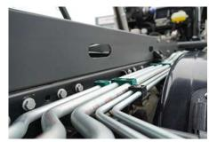
Power hydraulics can be set up in addition to the motion hydraulics, with connections at the rear right as standard, and pulled to the front as an option. Depending on the clutch, up to 52kW of power can be taken from the manual gear-box and up to 80kW from the reduction gearbox to drive other systems.
