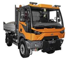
The maximum load capacity of **4,800 kg** and hydraulic relief at the front of the vehicle make the MT 770 a reliable partner for **demanding work**. The **total weight** is **7,500 kg**.
