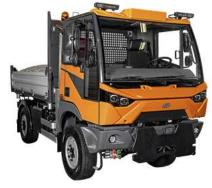
The maximum load capacity of **3,800 kg** and the extensive basic equipment of the MT 760 enable everyday use in all seasons. The **total weight** is **6,500 kg**.
