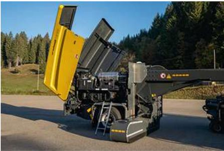
The drive motor drives the hydraulic pumps for operating and controlling the sweeping unit and blowing unit. The snow plough is controlled by a hydraulic system driven by the carrier vehicle's engine. The TJS/TJS-C's hydropneumatic chassis offers the operator additional comfort in the field.
