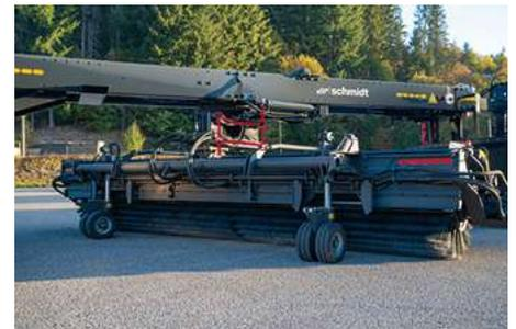
The twin castors offer very quiet, vibration-free and smooth sweeping performance, while level snow ejection and the cleanest fine clearing ensure maximum safety. This is achieved thanks to aerodynamic spoiler guidance, automatic spoiler adjustment and wear-dependent brush speed adjustment. This permits the jet sweeper to deliver a specific fine clearing result, while the robust design offers both optimum operational capability and maximum safety.
