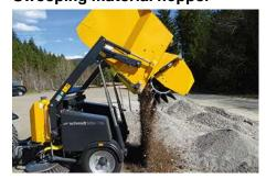
The MSH towed sweeper series has a steel hopper with a capacity of  $0.7~\rm m^3$  and a discharge height of 1,500 mm for the MSH 070 version and a capacity of  $1.5~\rm m^3$  and a discharge height of 1,800 mm for the MSH 150. In each case, the hopper is tipped hydraulically at the back.
