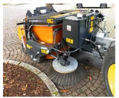
The MSH 070 has a steel hopper with 0.7 m³ capacity.
