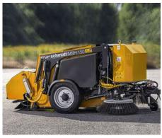
The MSH 150 has a steel hopper with 1.5 m³ capacity.
