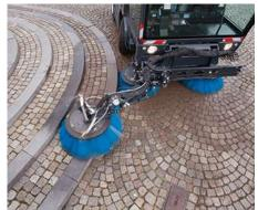
With the optional third brush, the working width can be increased to 3,550 mm. This allows a greater area output and sweeping on two levels.
