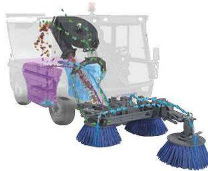
The 3-brush system with freely movable front brush arm offers a sweeping width of up to 2,600 mm. Left-right alignment of the front brush is just as possible as sweeping on two levels or heavy weed brush use.
