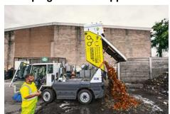
The hopper, which has a system volume of 2.6 yd³ (2 m³), enables maximum sweeping capacity and a large radius of action. The hopper is made of corrosion and saltwater resistant aluminium. A large dumping height of 55-1/8 inches (1400 mm) enables emptying into all common dirt containers. The suction pipe in the hopper is optionally available in wear-resistant stainless steel.
