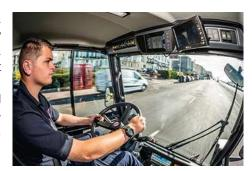
The most important information is visible at a glance on the **color display in the roof console**. With the help of the **onboard diagnosis system**, any faults can be localized quickly and efficiently, while a mechanic can make machine-specific settings on the display.
