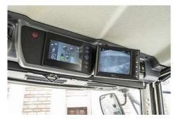
The sweeping unit is controlled via the door control panel with joysticks and push buttons. With the **Auto-Drive option**, all sweeping functions and driving commands in sweeping mode can be conveniently operated via the ergonomically shaped multifunctional control lever. Driving and sweeping from a single source also means greater safety and less stress.
