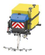
The CSP 3000 has a brine tank with a capacity of 3000 l.
