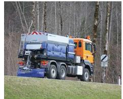
The Stratos RSP 50K Flex High has a hopper volume of 6.5 yd<sup>3</sup> with two integrated flex bags and is equipped with the RSP distribution system.
