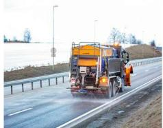
The Stratos WSP 50K has a hopper volume of 6.5 yd<sup>3</sup> and is equipped with the WSP distribution system.
