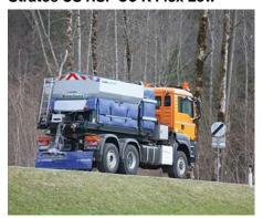
The Stratos RSP 50K Flex High has a hopper volume of 5.0 m<sup>3</sup> with two integrated flex bags and is equipped with the RSP distribution system.
