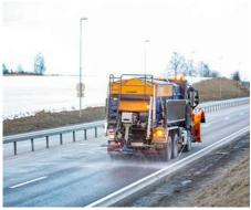
The Stratos WSP 50K has a hopper volume of  $5.0 \; \text{m}^3$  and is equipped with the WSP distribution system.
