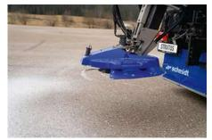
maintained, with a precisely defined spreading pattern and a spreading width of 2 - 10 m or 3 - 12 m. New in the range are the Premium PW50 spreading discs which allow a 2 - 6 m or 2 - 8 m width to be spread with an PW50 mix.
