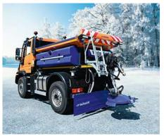
The Stratos F25 is a flat silo spreader with a hopper capacity of 2.5  $\mbox{m}^3.$
