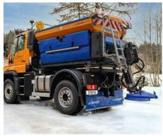
The Stratos 25 is a silo spreader with a hopper capacity of  $2.5 \text{ m}^3$ .
