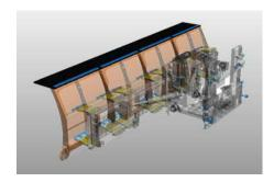
3. an adjustable snow deflector made of cloth. This version is particularly suitable for powder snow and high speeds
