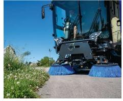
A flexible sweeping system helps ensure thorough cleaning in any situation. The towed disc brush system, mounted in front of the front axle, achieves a sweeping width of 86.6 in.
