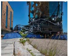
With the optional third brush, the working width can be increased to 3,550 mm. This enables a greater area coverage and sweeping on two levels.
