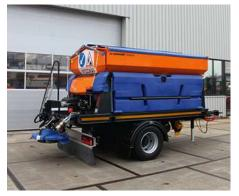
The Stratos A50K is a trailer spreader with a hopper capacity of 5 m<sup>3</sup>.
