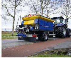
The Stratos A50K is a trailer spreader with a hopper capacity of 6.5 yd<sup>3</sup>.
