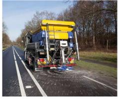
The Stratos 50 is a mounted spreader with a hopper capacity of  $6.5 \text{ yd}^3$ .
