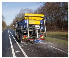
The Stratos 50 is a mounted spreader with a hopper capacity of 5 m<sup>3</sup>.
