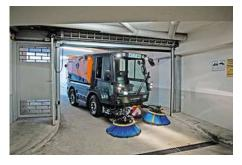
A lowerable running gear (optional) simplifies driving in multi-storey car parks and low entrances. The chassis can be lowered by around 70mm at the push of a button and the system levels itself automatically.
