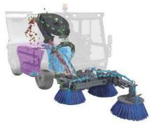
The 3-brush system with freely movable front brush arm offers a sweeping width of up to 2,600 mm. Left-right alignment of the front brush is just as possible as sweeping on two levels or heavy weed brush use.
