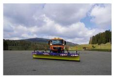
When fully unfolded, the snow plough has an outstanding working width of 6.2 m. When the left wing is folded in, the working width reduces to 5.1 m, and when the right wing is folded in, it reduces to 4.5 m. When both wings are fully folded, the clearing width is 3.4 m, while the wings can folded hydraulically in both transport and clearing positions, minimising the transport width. They are automatically raised during the clearing operation.
