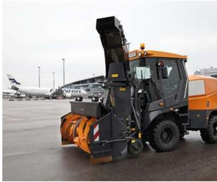
The Supra 5002 is a self-propelled snow clearing machine with a clearing width of either 2400, 2600 or 2800 mm. It is particularly recommended for airports with a clearing capacity of up to 5,000 t/h
