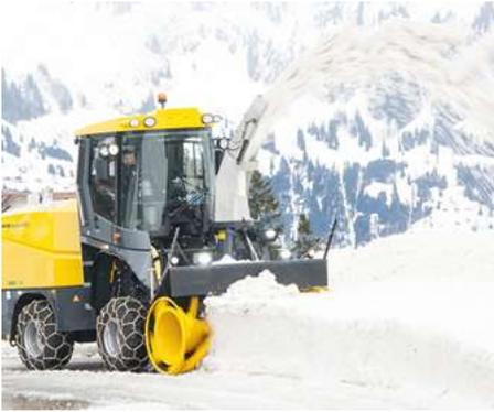
The Supra 4002 is a self-propelled snow clearing machine with a clearing width of either 2400 or 2600 mm. With a clearing capacity of up to 3,500 t/h, it is ideally suited for pass and road clearing.
