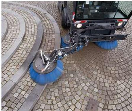
With the optional third broom, the working width can be increased to 3,550 mm. This allows a greater area output and sweeping on two levels.
