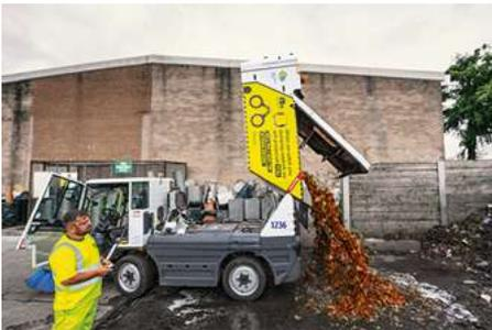
The hopper, which has a system volume of 2m<sup>3</sup>, enables maximum sweeping capacity and a large radius of action. The hopper is made of corrosion and seawater resistant aluminium. A large dumping height of 1400mm enables emptying into all common dirt containers. The suction pipe in the hopper is optionally available in wear-resistant stainless steel.
