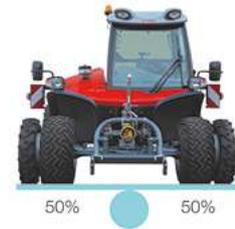
**Torsen / T-Traction:** The Torsen centre differential ensures continuous distribution of the drive torque to all four wheels. This protects drive components and wheels, while also being easy on the ground. The optionally available T-Traction prevents front or rear wheels with no appropriate counterweight from slipping in challenging situations.
