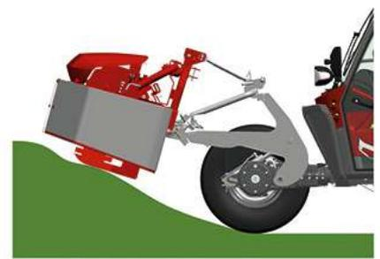
**Terrain adjustment:** The front axle can rotate against the rear, aligning the machine to the terrain with absolute precision. The integrated skew suppression works progressively until it stops.
