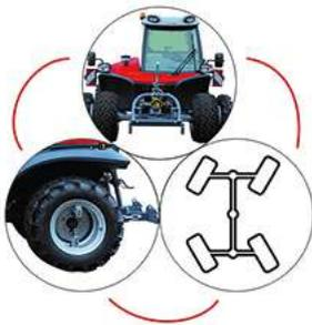
**Smart work with automated processes:** The intelligently interlinked technology automatically turns on the all-wheel steering system and lifts the rear hoist as soon as the front hoist is lifted. This saves you time and allows you to work smarter.
