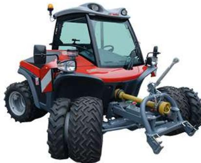
The powerful turbo diesel engine of the **Aebi TT 211** has an output of 53 kW (72 PS) and a high torque, which is already reached at 1500 rpm. The requirements to the exhaust gas stage V are far exceeded by the turbo diesel engine in the Aebi TT 211.
