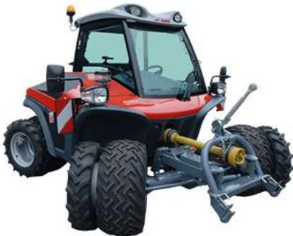
The diesel engine of the **Aebi TT 206** has an output of 42 kW (57 hp), a strong torque increase and meets the high requirements to achieve exhaust gas stage V. The highest torque is already reached at 1600 rpm.
