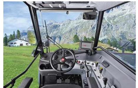
**A drive level without compromise:** Outstanding ergonomics, comfort and functionality, with pinpoint and ultra-quick instrument control with just one finger. A new drive lever with Smart Navigator is integrated into the armrest and allows for a relaxed posture in any situation.
