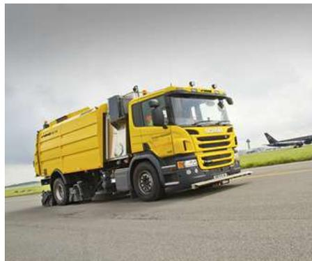
The AS 990 series machine can also be equipped as a stand cleaning machine. The stand cleaning option is particularly suitable for collecting rubber abrasion and oil.
