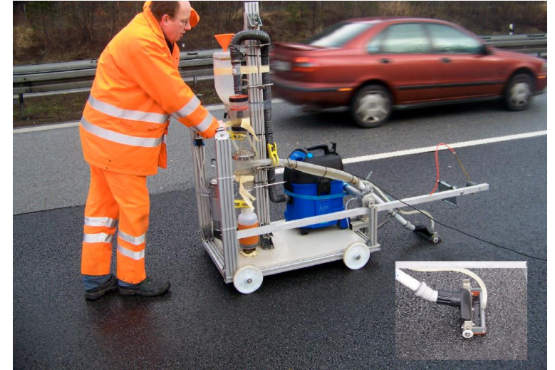
Measuring the amount of salt using sensors (test field, 12 sensors)
