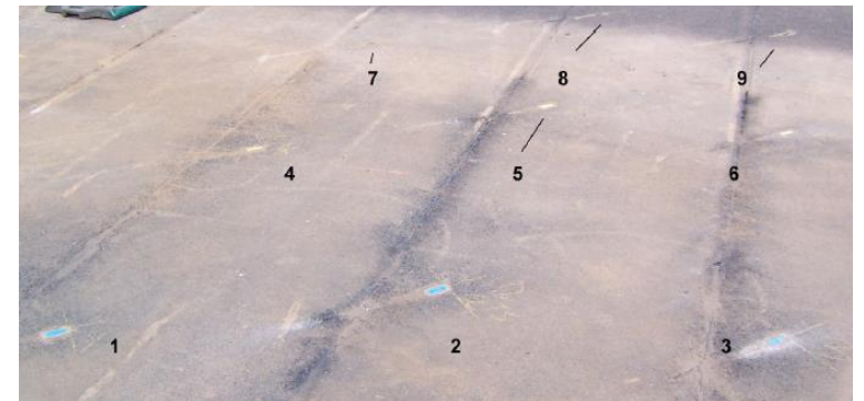
Measuring the amount of salt using sensors (test field, 12 sensors)
