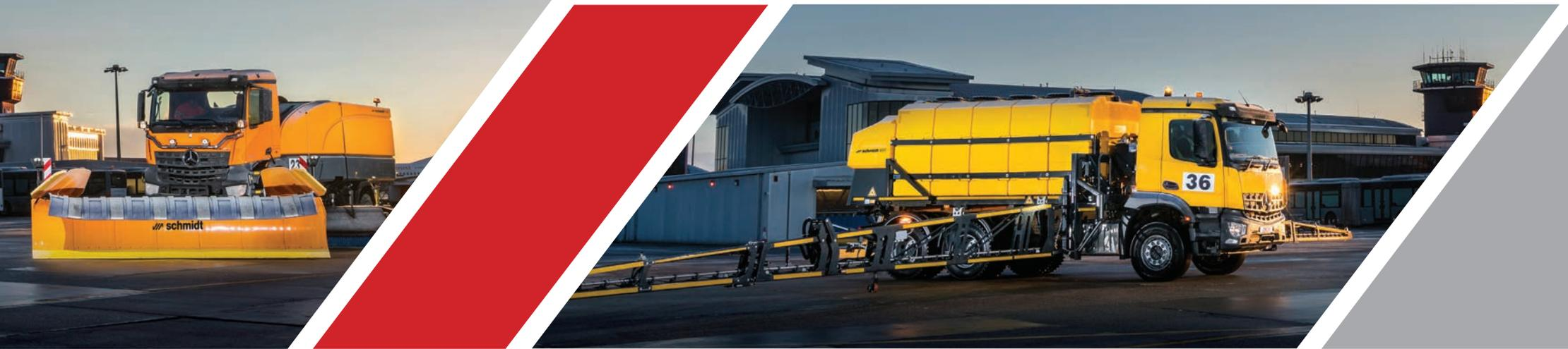
Designed specifically for keeping runways clear and ice-free, the ASP is available as both a fix-mounted or demountable variant for trucks, operating at speeds of up to 30mph and with spraying widths ranging from 3-30m.
