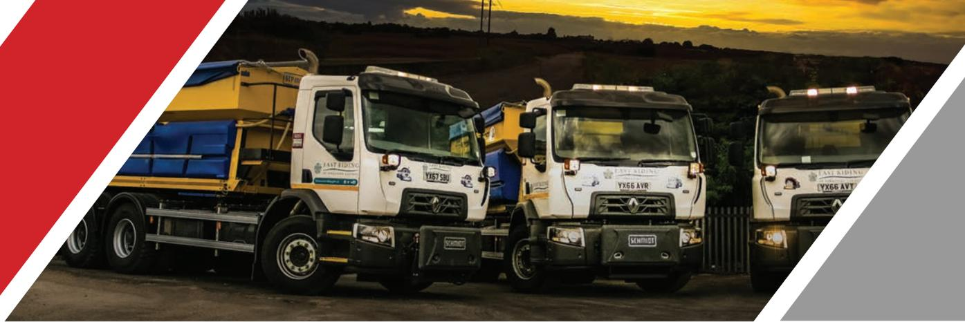
The Council runs a fleet of 21 9m<sup>3</sup> vehicles and has just ordered a batch of 5 new Stratos III 9m<sup>3</sup> spreaders mounted on Renault chassis to replace existing equipment that has come up for replacement and will shortly be de-fleeted.
